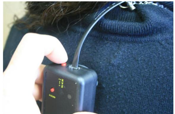
Instruct the patient to follow the instructions on the screen. **Press the red button when the patient reaches their maximum position away from neutral.** The angle difference between the two inclinometers (their true extension angle) appears in circle #1. If computer speakers are enabled, a “beep” sounds, indicating a recorded reading. Instruct the patient to return to slightly beyond their starting neutral position (i.e. after tilting their head back to their maximum, instruct them to move
